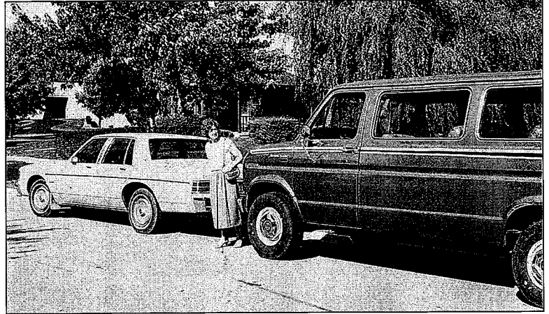
FIGURE 9-1. On-street parking typically results in less visibility between motorists and pedestrians.
