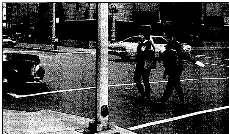
FIGURE 6-5. Standard marked crosswalks of two parallel lines are commonly used but are not as visible as ladder or other "high visibility."
