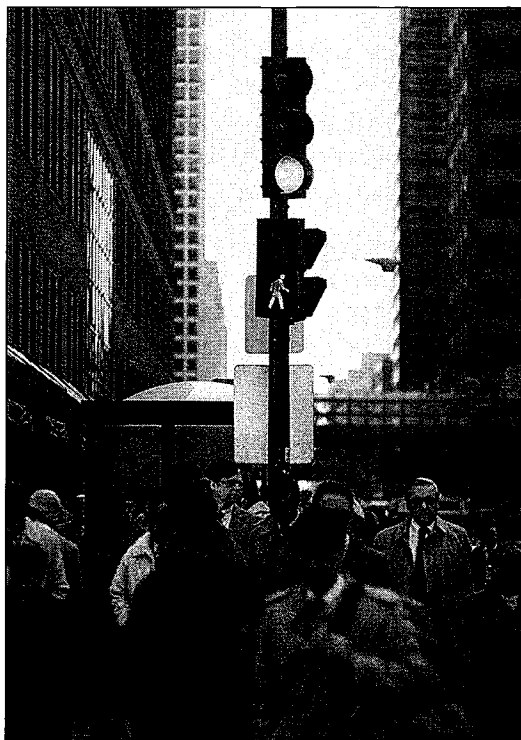
FIGURE 5-5. The MUTCD recommends at least a 4-to 7-second walk interval, but a longer interval is desirable.
