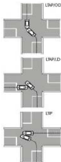
Figure 1: Conflict Points for a Left Turning Vehicle at an Intersection
