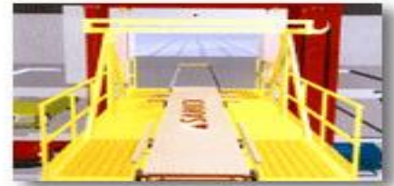
Trolley returned the platform after locating the vehicle
