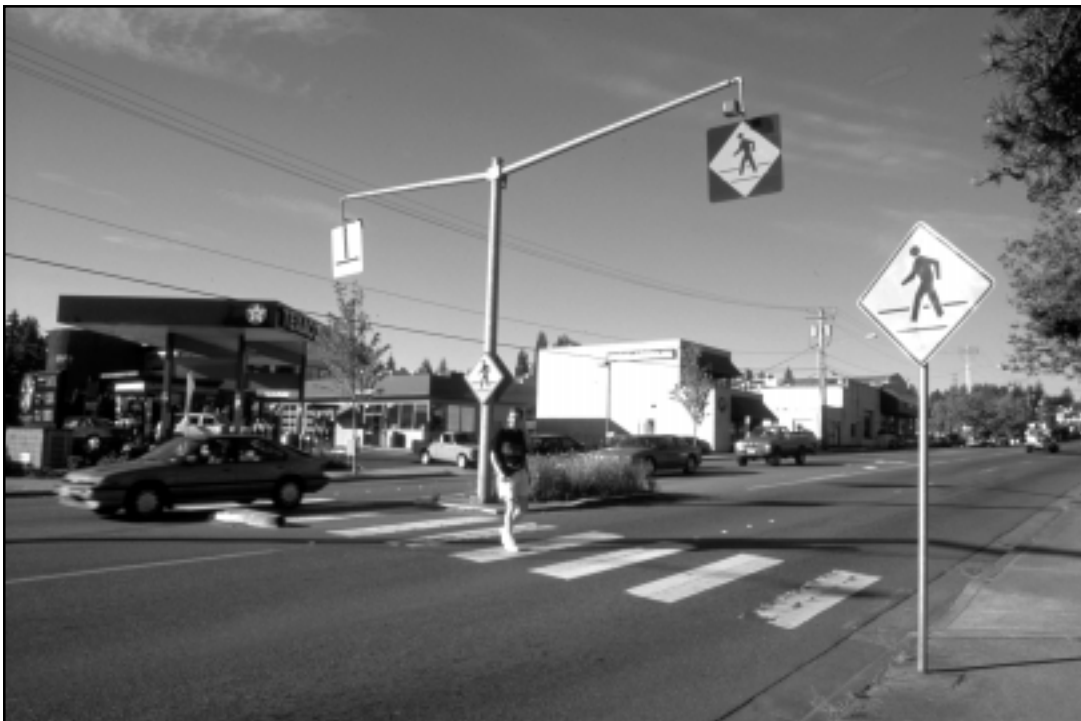
Figure 7-3. Pedestrian crossing signs along the edge of the roadway may be supplemented by signs in the median, overhead signs, and high-visibility crosswalk markings.
