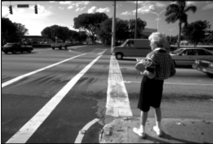
Figure 11-3. Signals frequently used by elderly or physically impaired pedestrians should be retimed to provide a crossing time commensurate with their ability.
