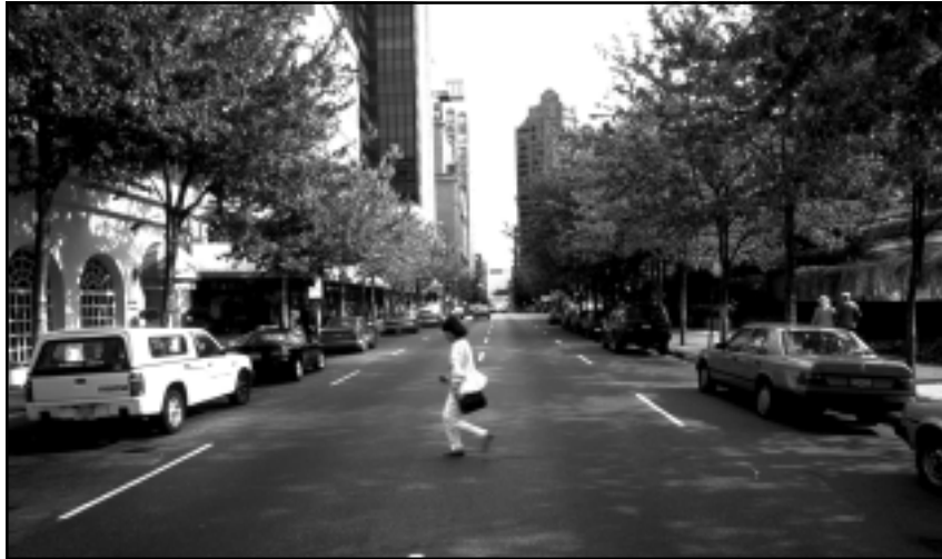
Figure 10-2. One-way streets that contain wide travel lanes can result in higher than desired vehicle speeds, which can cause problems for pedestrians.
