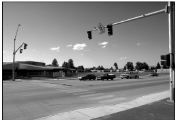
Figure 9-7. The failure to use stop lines encourages many motorists to stop too close to the intersection, forcing pedestrians into the parallel roadway. A midblock stop line queues motorists back 40 feet, reducing the chance for a multiple threat crash.
