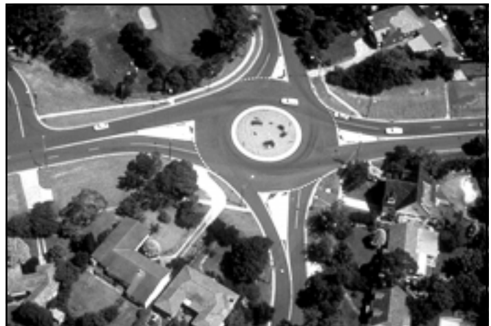
Figure 11-5. Modern roundabouts can reduce vehicle speed and pedestrian/vehicle conflicts.
