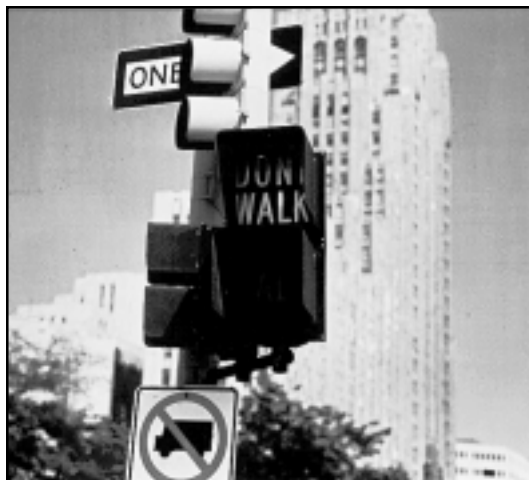
Figure 8-1. Pedestrian signal displays.
