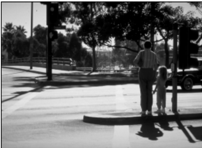
Figure 8-5. Pedestrian push button and signal heads are placed in channelized islands to guide pedestrians over a shorter crossing distance.
