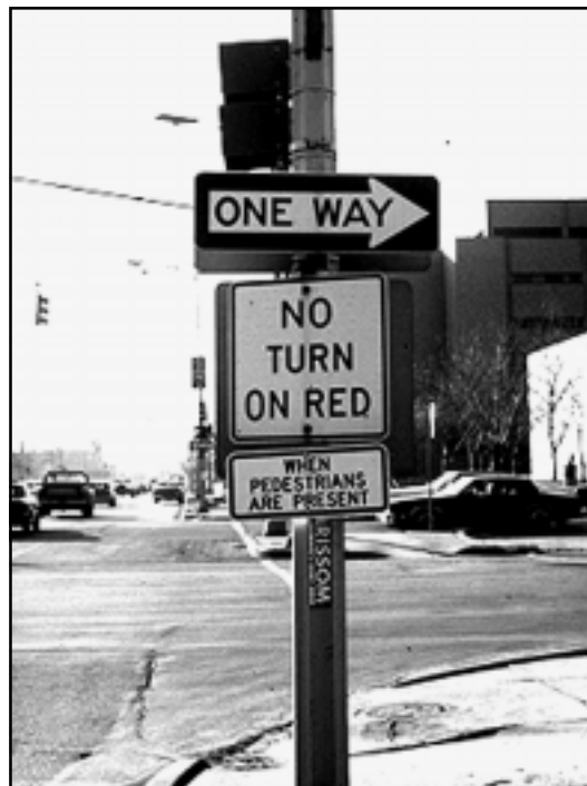
Figure 8-6. Right-turn-on-red restrictions can improve pedestrian safety when used properly. The top sign creates confusion and should not be used. The bottom sign conveys a much clearer message.
