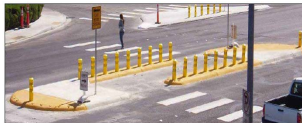
Raised Median with Offset Opening
