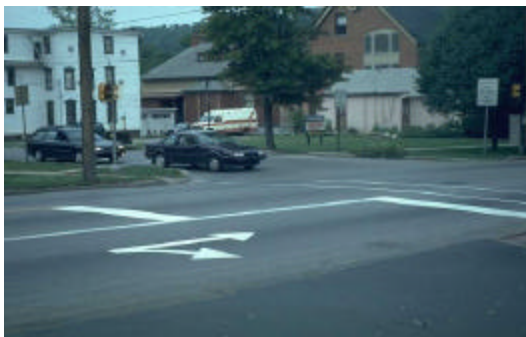
Recessed Stop Bar for traffic turning left
