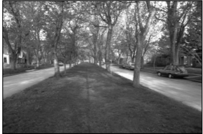
Figure 21-2. Neighborhood boulevard streets produce low-speed travel. Proper placement and undercutting of trees keep sight lines open.
