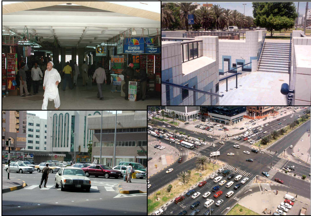
FIGURE 3 Examples of grade-separated and signalized pedestrian crossings
