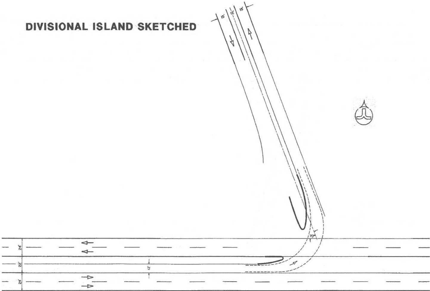
Figure 9-23. Channelization Developed From First Left-Turn Plot.
