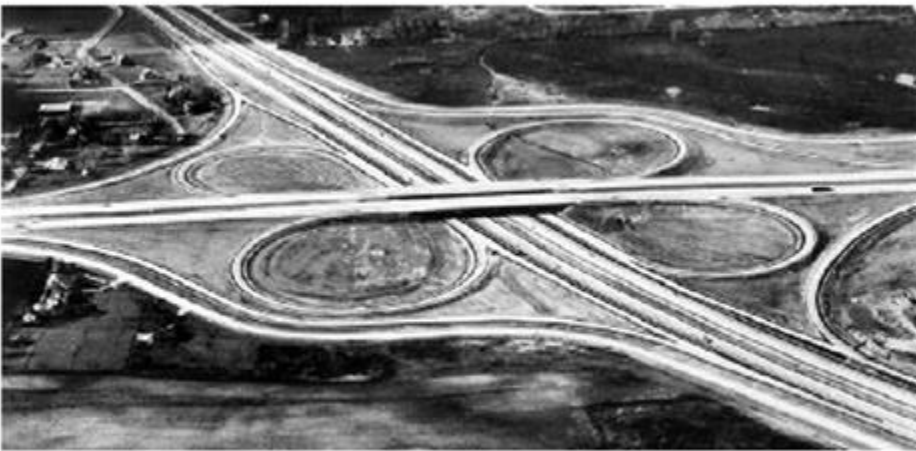
Exhibit 10-26. Four-Leg Interchange, Full Cloverleaf With Collector-Distributor Roads
