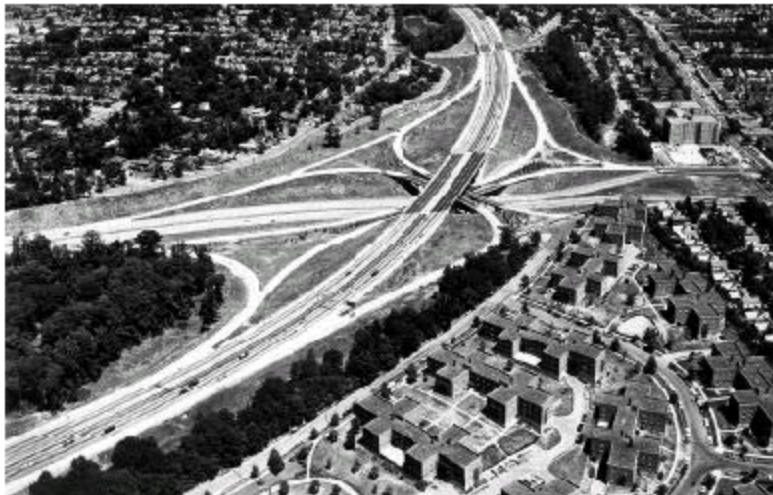
Exhibit 10-35. Four-Level Directional Interchange
