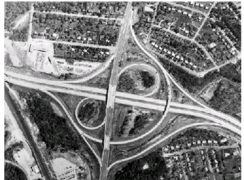
Exhibit 10-37. Semidirectional Interchange With Loops
