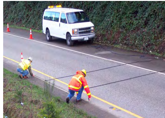
Short Duration Traffic Collection Field Crew Setting Road Tubes
