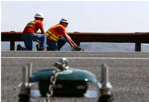
New Technology – Infrared Traffic Loggers - TIRTL
