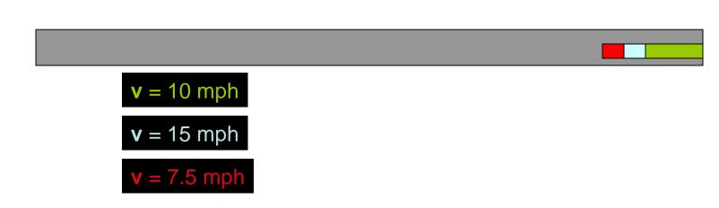
Average speed measured by TMS and SMS is different even though the individual bike speed are exactly the same
